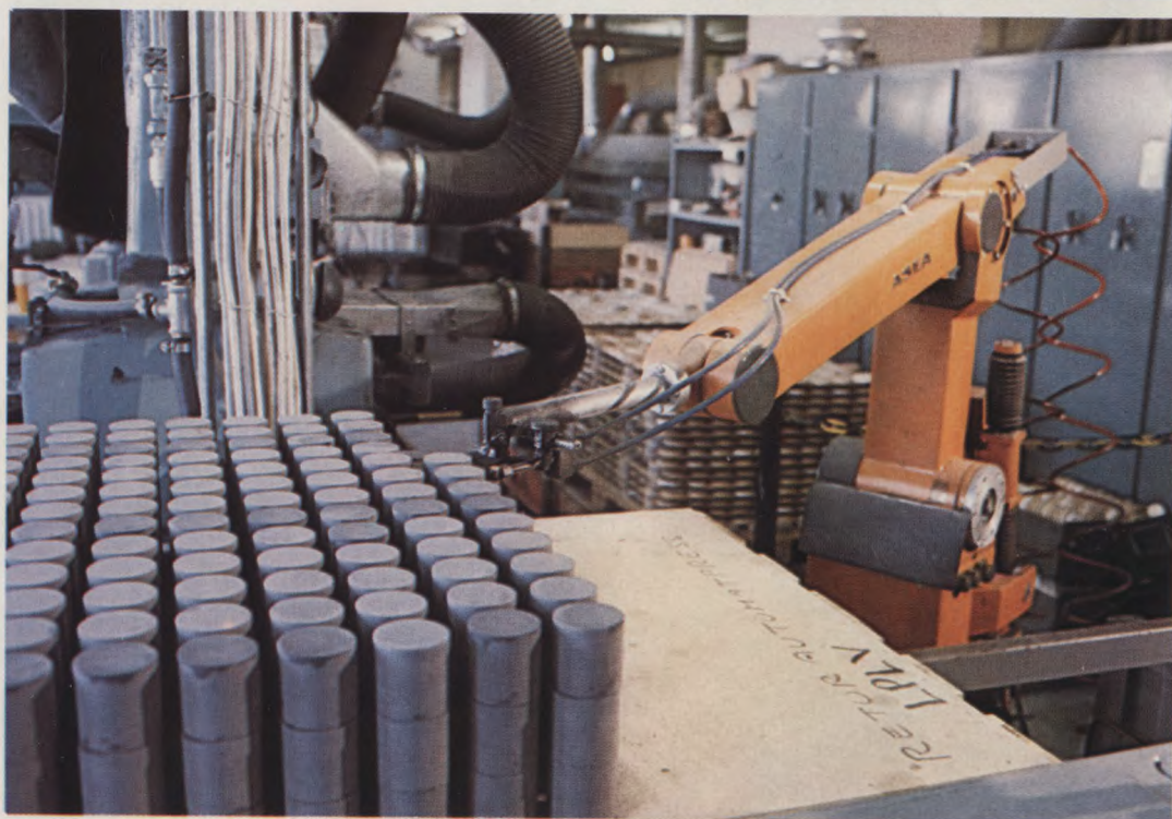
Example of pattern laying. The pattern-laying function includes: a program for picking items from a press common for all items. A separate program section for each put-down position. (F 93373)
