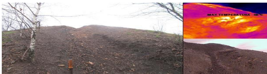
Fig. 5.25. Motorsports and cycling on dump leads to creation of erosion trenches, which help providing oxygen to waste mass that is necessary in self-heating processes [source: own]
