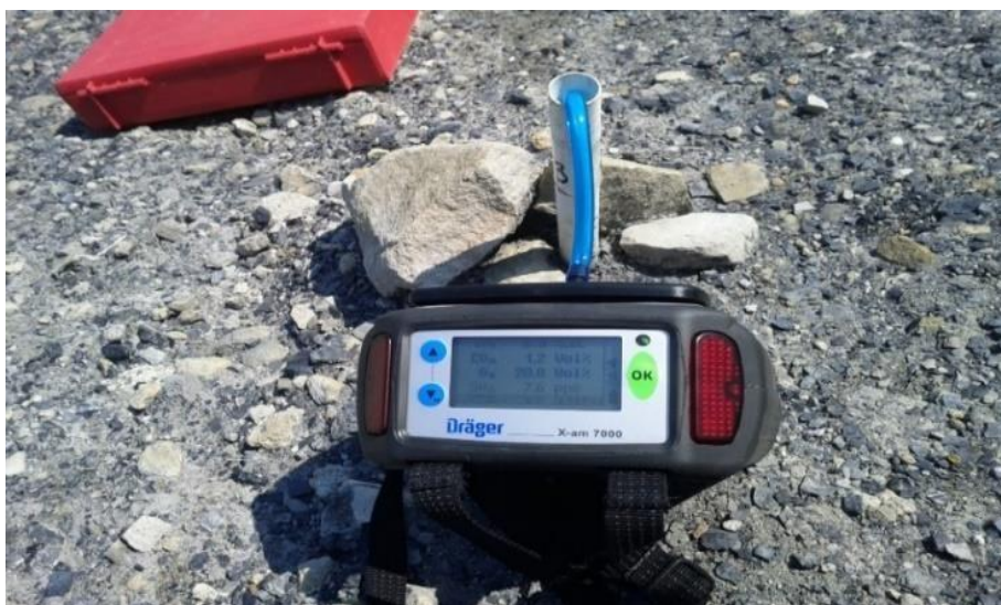
Fig. 5.11. Measurement of gas concentration using Dräger X-am7000 detector
